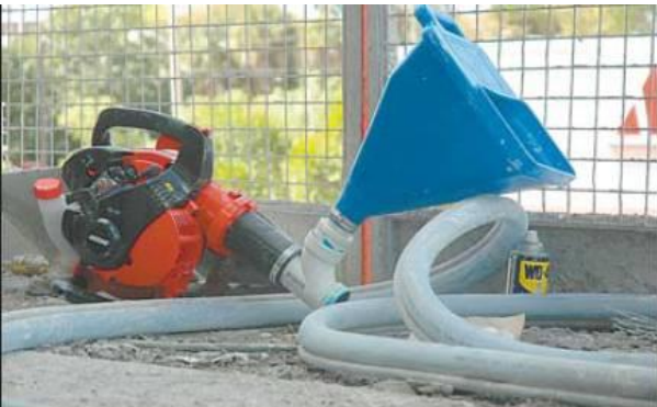
Above, a worker blows on the wet final coat, which is then troweled and blown with shell from this blower/hopper combination, below.
